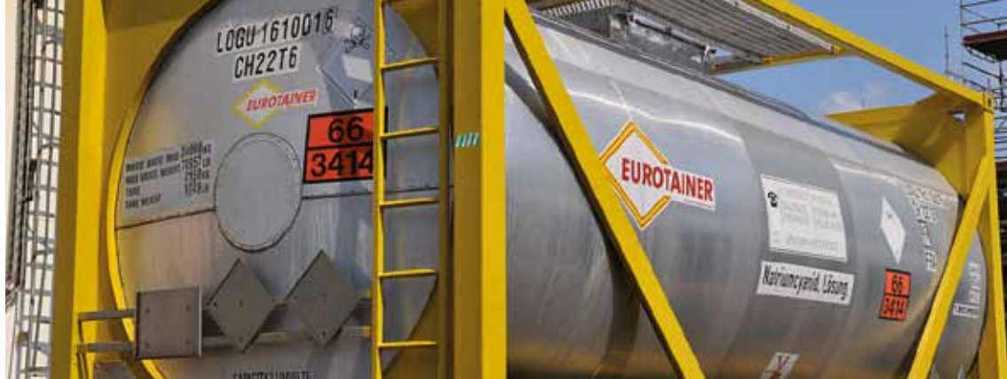
Photo: Cyanide container in a modern gold ore process plant
